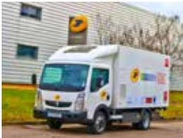
The Maxity Electric is an electric lorry equipped with a hydrogen-powered range extender, which doubles autonomy to 200 km in comparison with standard lorries. It was developed by Renault Trucks in partnership with Symbio FCell, and is currently being tested under real roadway conditions by the French postal service.
